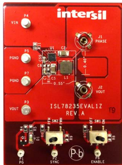
FIGURE 1. ISL78235EVAL1Z EVALUATION BOARD PHOTO
